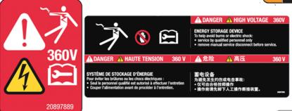
The high voltage danger labels are red and indicate that high voltage is present at all times. These labels are located on the high voltage battery.
