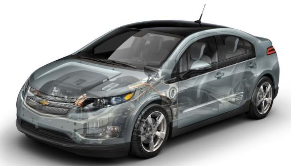
The Chevrolet Volt is a front-wheel drive, four-passenger electric vehicle with extended-range capability. The vehicle is propelled exclusively by electric motors. The Volt uses high voltage energy that is stored in the high voltage battery as its primary power source. However, once the battery capacity is reduced, the gasoline engine drives a generator which produces electricity to power the vehicle.
